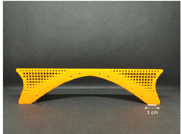
Fig. 8: Simply-supported beam with a distributed load of Fig. 6d printed using FDM 3D printer.
