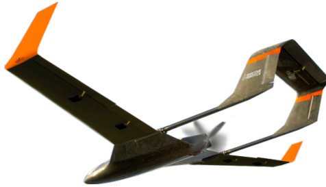
Figure 7.7: P31016 concept battery-powered fixed-wing unmanned aircraft
