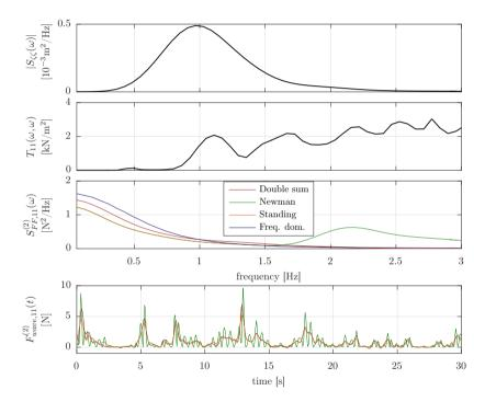
Figure 1.3 Wave spectrum (top), mean drift coefficients  $T_{11}(\omega, \omega)$ , surge slow-drift force spectrum  $S_{FF,11}^{(2)}(\omega)$  and time series  $F_{11}^{(2)}(t)$  with frequency-domain calculation (Eq. (1.31)), double IDFT (Eq. (1.32)), original Newman approximation (Eq. (1.33)) and Standing et al.'s formulation (Eq. (1.34)), from [24].
