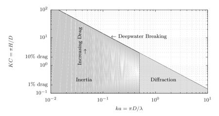
Figure 1.2 Wave-induced force component domains. Taken from [24], originally from S.K. Chakrabarti.
