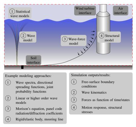
Figure 1.1 Hydrodynamic Modeling of the Offshore Wind Turbine System.
