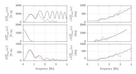
Figure 1.4 Morison excitation transfer functions  $G_{Fmor}(\omega)$  for Froude-Krylov component only (blue) compared to panel code transfer functions  $\mathbf{X}(\omega)$  (orange), from [24].
