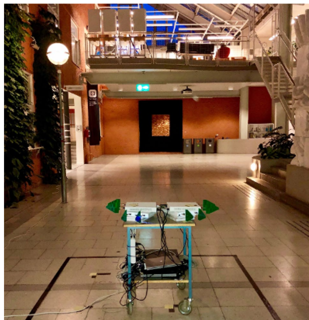
Fig. 3 Positioning of the base station on the balcony and the user equipment cart. The antennas are pointing away from the balcony to illuminate non-line of sight links. Five physical locations in the black square were measured for each frequency band
