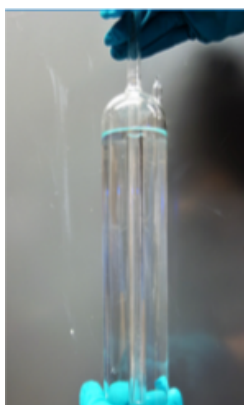
Figure 3.7: Triple point cell for water.
