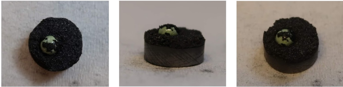
Figure 4.4.1.2: Pictures of slag drop and coke pellet after test 14
