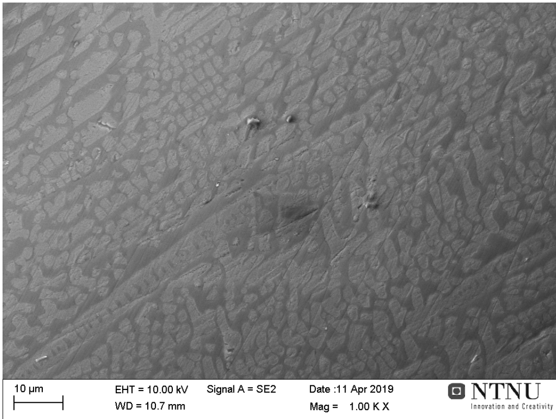
Figure 4.4.4.6: Details of two-phased slag of sample 17 magnified 1000 times
