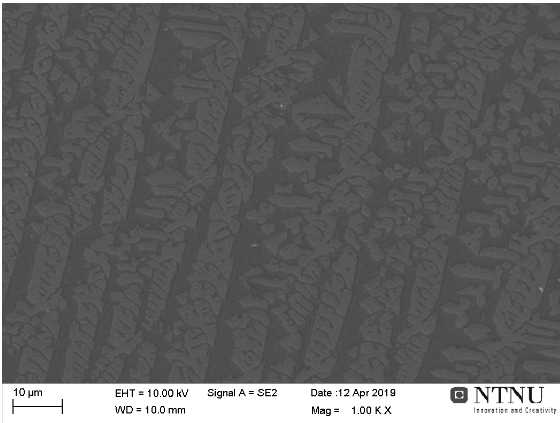
Figure 4.1.4.7: Larger two-phase slag of sample 5 magnified 1000 times
