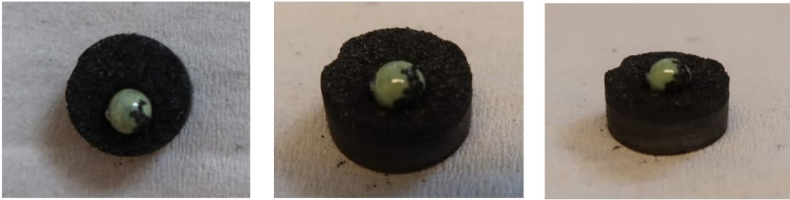
Figure 4.3.1.2: Pictures of slag drop and coke pellet from test 2
