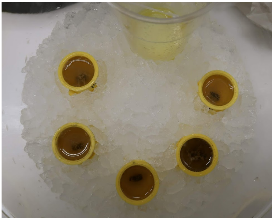
Figure 3.12: Samples in ice bath during iodine epoxy casting
