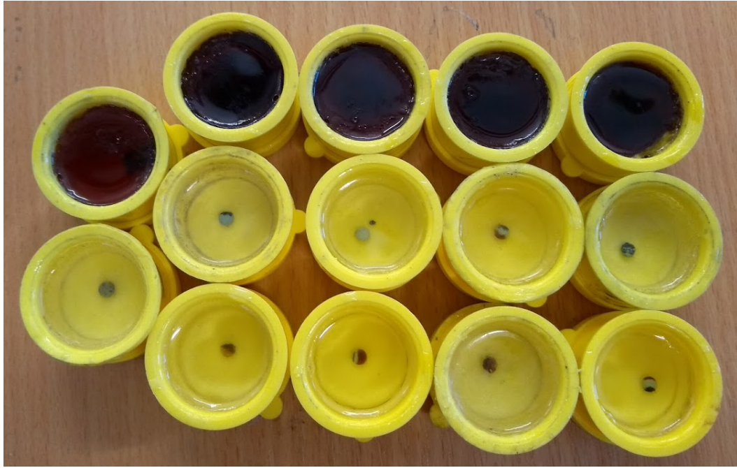
Figure 3.13: Hardened samples, nine in epoxy and five in iodine epoxy.
