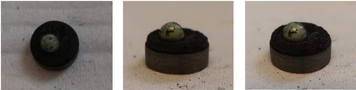
Figure 4.1.4.2: Pictures of slag drop and charcoal pellet after test 5
