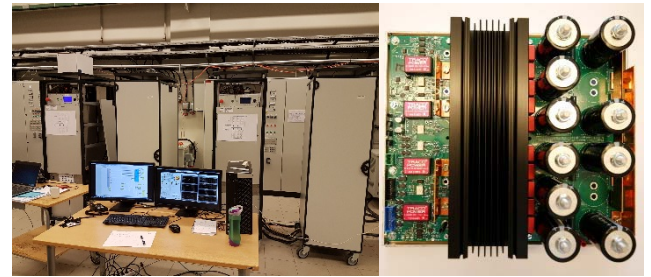
Fig. 4. Overview of laboratory setup and picture of circuit board with two half-bridge sub-modules
