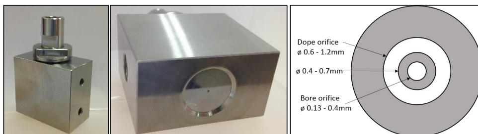
Figure 4.1: Spinneret photos (left) and range (right) of different dimensions used for spinning of CAHF
