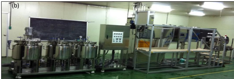
Figure 4.2: (a) Schematic diagram of hollow fiber spinning process (b) Photograph
