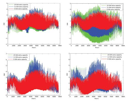
Fig. 2 Average production hour-by-hour in 79\_no (upper row) and 81\_no (lower row) with increased hydropower capacities for 75 simulation years, EMPS (left) and SOVN (right) results
