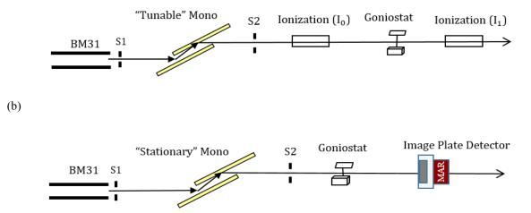
**FIGURE 2.** These are two experimental setups at BM31, SNBL. (a) depicts schematically the energy scan, (b) is the fixed wavelength  $\omega$ -scan setup which is used for orientational measurements.
