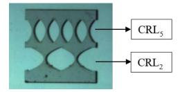
FIGURE 1. This optical photo of the planar lenses.
