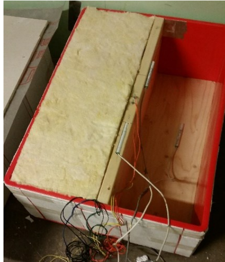
Fig. 2. Test box showing wooden joist, plywood (to the right) and measurement sensors before installation of SVB and gypsum board.
