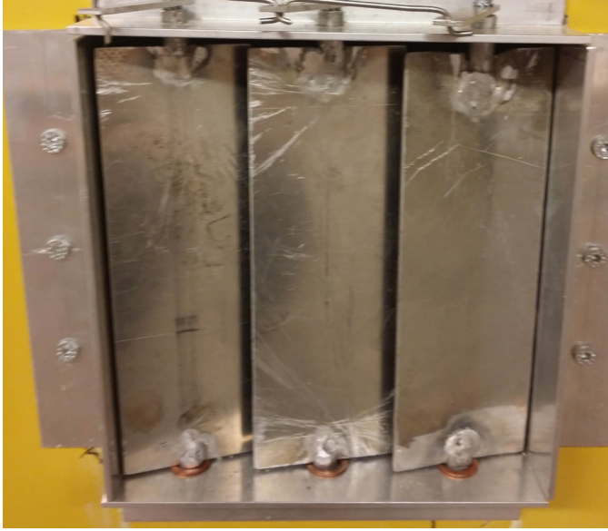
Fig. 4. Vent valves on scale model A.
