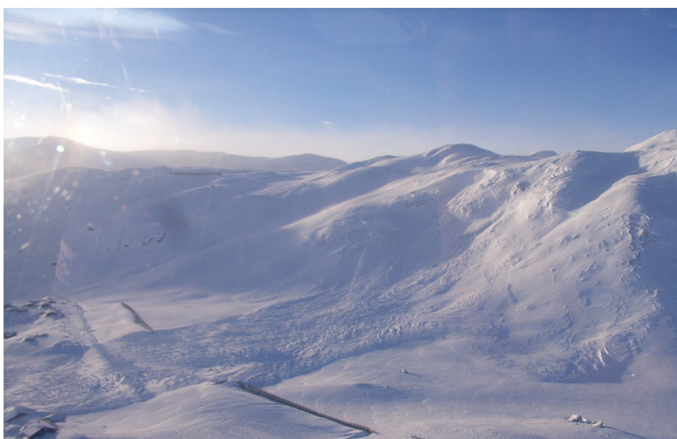
Figure 3.3: A large avalanche crossed the road and also hit buildings at Tyinstølen in January 2008. The runout length were over 600 m, despite a height difference of only around 170 m (Håland et al., 2015). The survey area called Tyinstølen in this study cover the left part of the release area seen on the picture. (Svein Helge Frækaland/NPRA)
