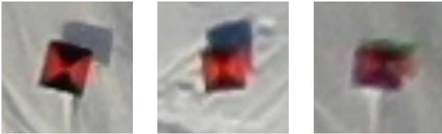
Figure 4.4: Differences in image quality shown by zooming in on GCP target plates (see figure 3.5). Left: Well contrasted and little visible distortion, from near image center. Middle: Clear image blur, from near image center. Right: Significant image blur and distortion, from near image corner.
