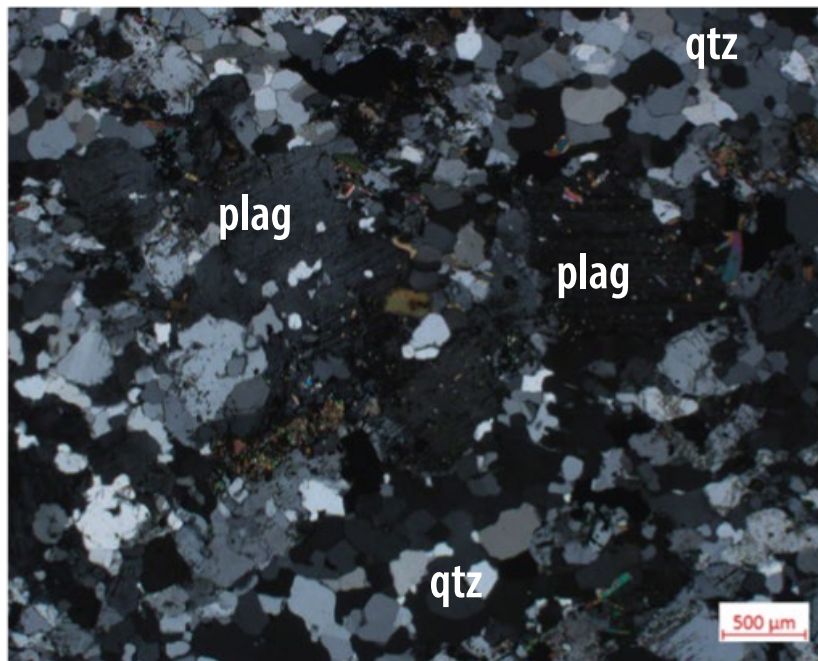
Microphotograph (XPL) showing saussuritization of plagioclase grains, and recrystallizing texture of quartz.
