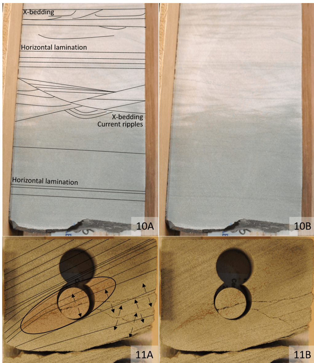
Figure 8.20: 10A is a proposed interpretation of 10B (sample 11) and illustrate both the planar laminated and the cross-bedded facies. 11A and 11B show the cross-bedded facies. 11A is an interpretation of 11B (sample 6).
