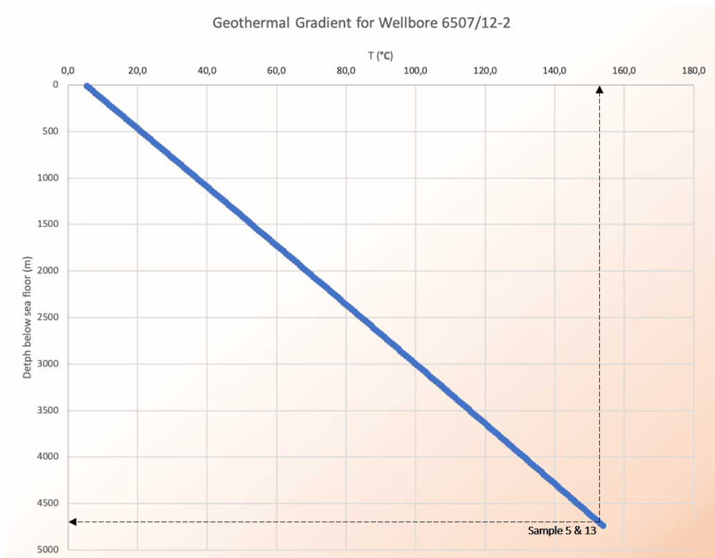
Figure 8.22: Geothermal gradient for well 6507/12-2. The depth from RKB to the sea floor is 286 m, and has to be added to the depth to get the MD.
