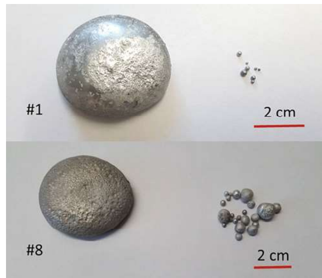
Fig. 6 Coagulated and non-coagulated droplets after recycling (Trial 1 and 8)
