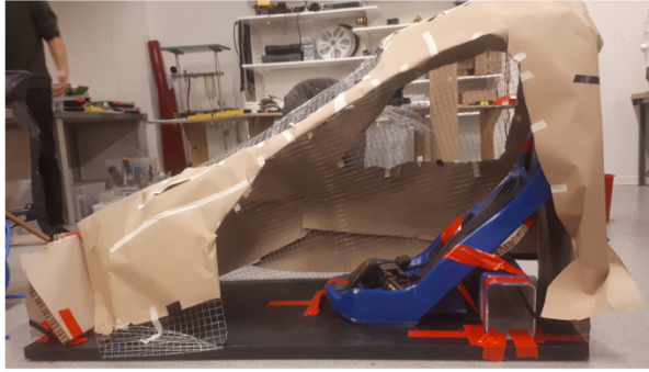
Figure 7: Left; the wire netting prototype, right; the minimum volumes determined by the prototype in CAD
