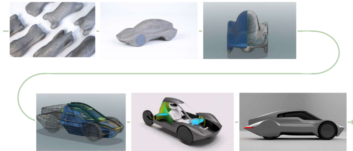
Figure 16: Several clay concepts were created initially (1-2), and were transformed into a 3D representation (3). The constraints and body were iterated multiple times for different T-spline representations (4-5), and design features were shaped using both 3D modelling and clay modelling (6)
