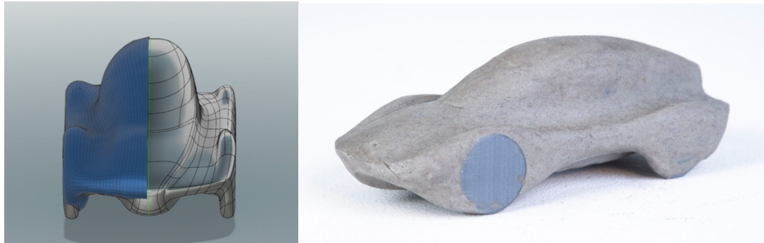
Figure 23: Left; the generated T-spline model (blue) and the initial constructed t-spline model. Right; the new clay model.
