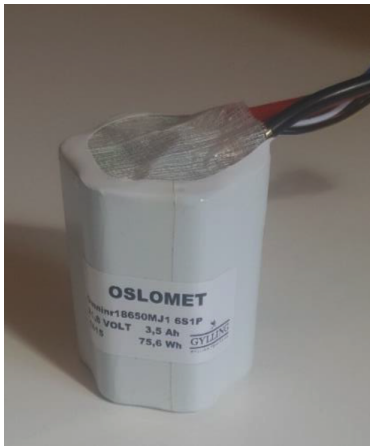
Fig. 4: Battery pack, lithium ion 6S 3500mah.
