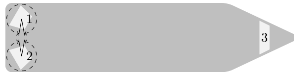
Fig. 2. Thruster configuration for vessel, where 1 and 2 are azimuth thrusters, and 3 is a tunnel thruster.
