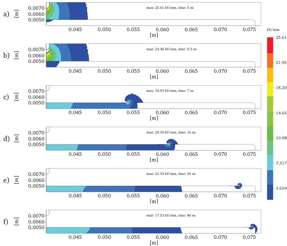
Figure 5.17: Simulation: electric field strength, applied 35 kV. The field is only plotted in regions where |\mathbf{E}| \geq 2.6 kV/mm, to visualize the position of the streamer head. The maximum field strength in air is located at the streamer head (value of maximum field strength indicated in each plot). The streamer slows down as it propagates into low background field regions. a) t = 0 ns (background field), b) t = 0.3 ns (streamer initiated from the blade tip, propagating towards the barrier), c) t = 7 ns (streamer propagation along barrier) d) t = 16 ns, e) t = 59 ns, f) t = 80 ns (streamer at the barrier edge). Entire simulation domain shown in fig. 4.5b.
