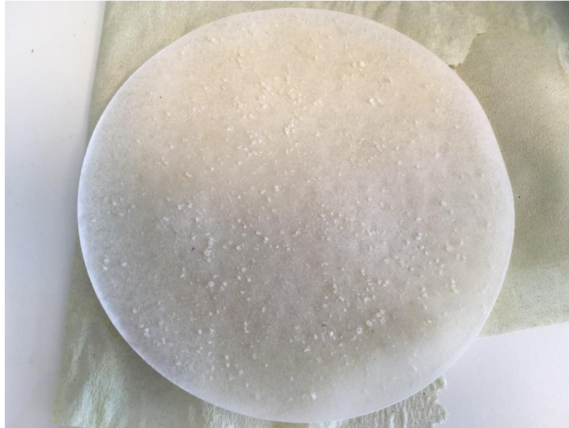
Figure 18: Particles retained by microfiltration in laboratory scale.
