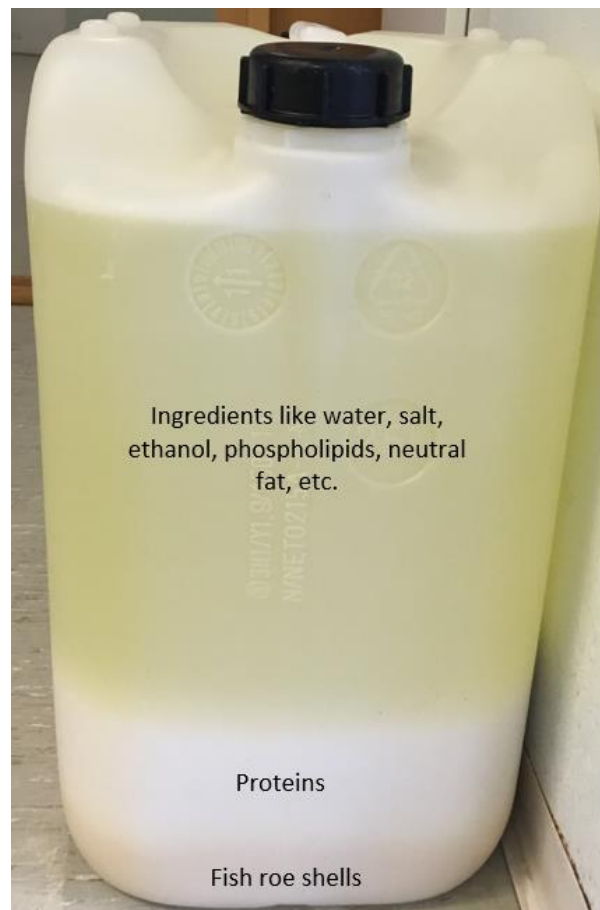
Figure 16: Dehomogenized mixed fish roe with solvent.
