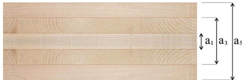
Figure 3.11: a_1 , a_3 and a_5 illustrated for a generic 5-layer CLT element
