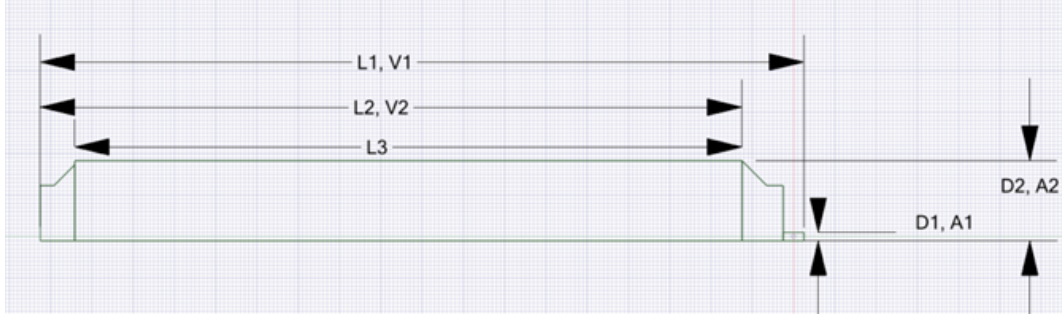
Figure 3.2: 2D sketch of the computational domain with measuring lines and parameters that was used in the first three cases.
