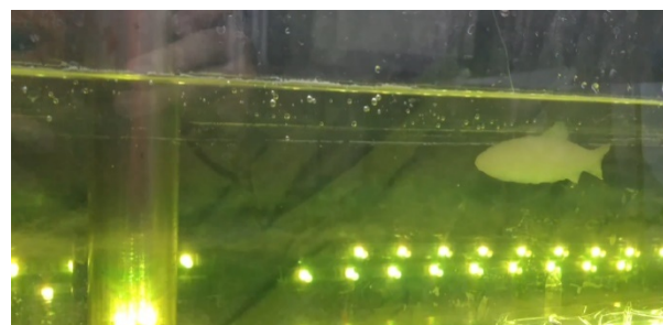
Figure 2: Rubber silicone fish suspended behind metal tube to replicate Kármán like swimming motions.
