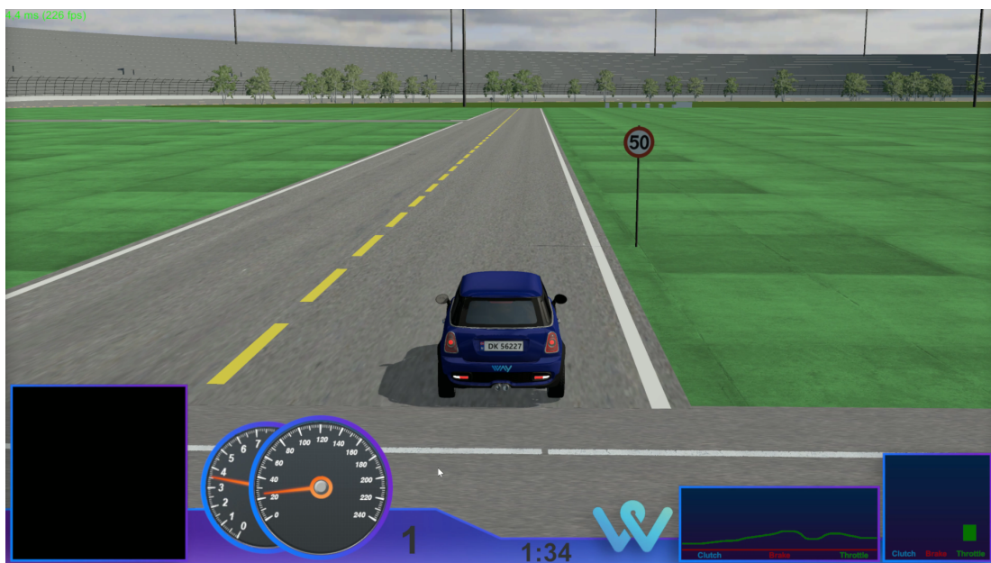
Figure 7.8: Initial acceleration is very high initially when cars spawn within the simulator, resulting in a possible collision and the system saying the Ego violates having to yield. In this case, the car is not seen, but is at the end of the road, in the lane opposite to the Ego.
