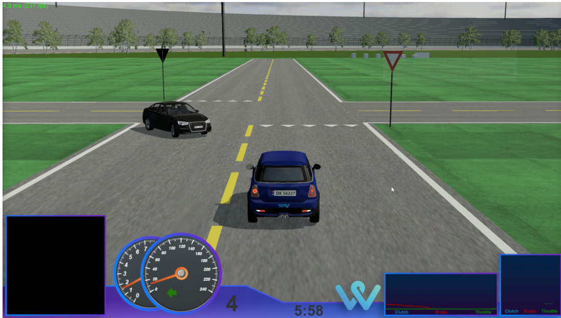
Figure 7.10: In scenario 9, the other car is on a collision path with the Ego, but the system says the Ego violates having to yield.
