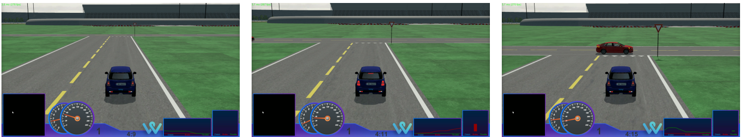
Figure 7.4: This example of scenario 6 shows the Ego not yielding when supposed to and having to compensate by braking hard. In this case, the proof of concept system provides feedback about violation of having to yield.
