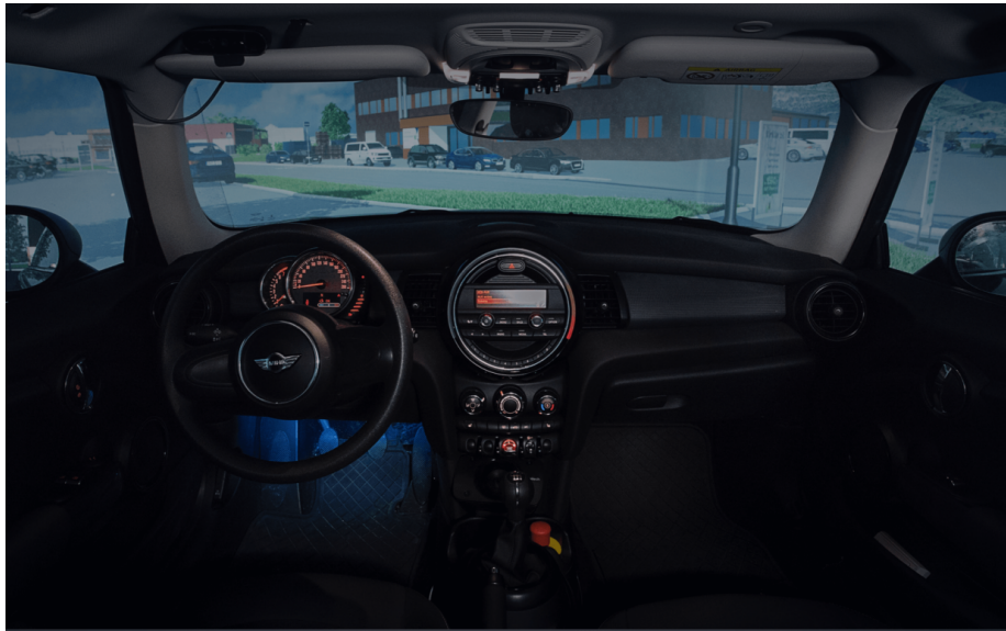
Figure 1.1: A picture taken from within one of Way AS' driving simulators. There is no physical engine, input actions from the car are instead applied within the virtual simulator world.
