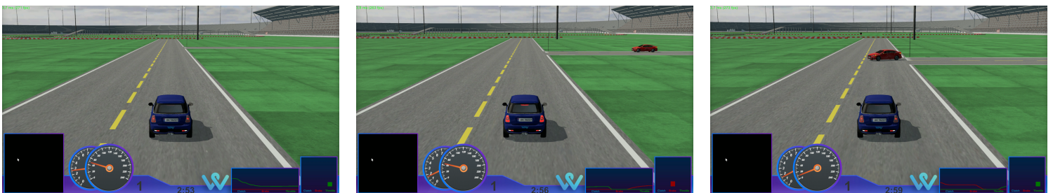
Figure 7.7: This example of scenario 4 illustrates stopping to let another car having to yield for you pass, in the case of having right of way. In this case, the proof of concept system provides no feedback as there were no violations of having to yield.
