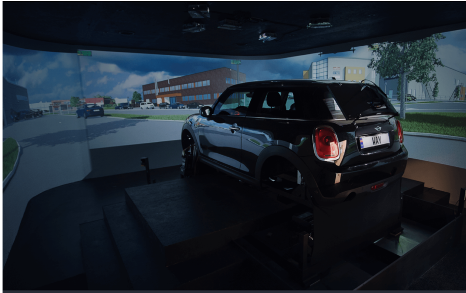
Figure 5.1: A picture taken from within one of the rooms in which Way AS has a driving simulator. A car is driven as normal, without the engine running, and wheels turning, but the driver input is emitted onto a local network. The resulting actions are performed in the simulator world, and the world is projected 360 degrees around the car, as well as to a screen in the rear view window.
