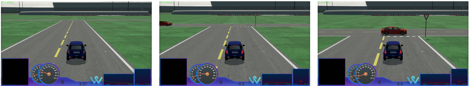
Figure 7.5: This example of scenario 6 shows the Ego yielding when supposed to, by adjusting speed appropriately beforehand. In this case, the proof of concept system provides no feedback as there were no violations of having to yield.
