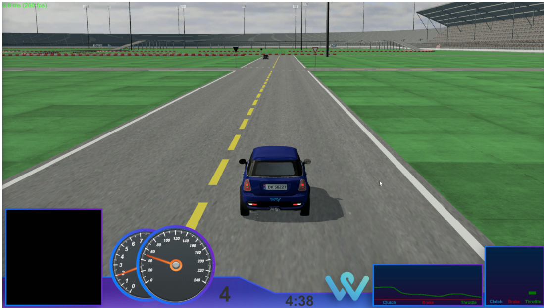
Figure 7.9: Adjustment of ones position in the lane, due to the intended path, is an over-sensitivity within the system that results in the system saying the Ego violates having to yield.
