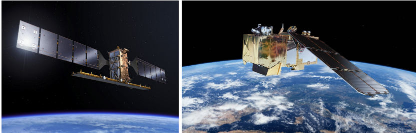
Figure 2.6: Sentinel-1B and Sentinel 2. Two ESA satellites used for remote sensing. Sentinel-1B uses active radar technology to observe the Earth, while Sentinel-2 uses a passive multispectral sensor.
