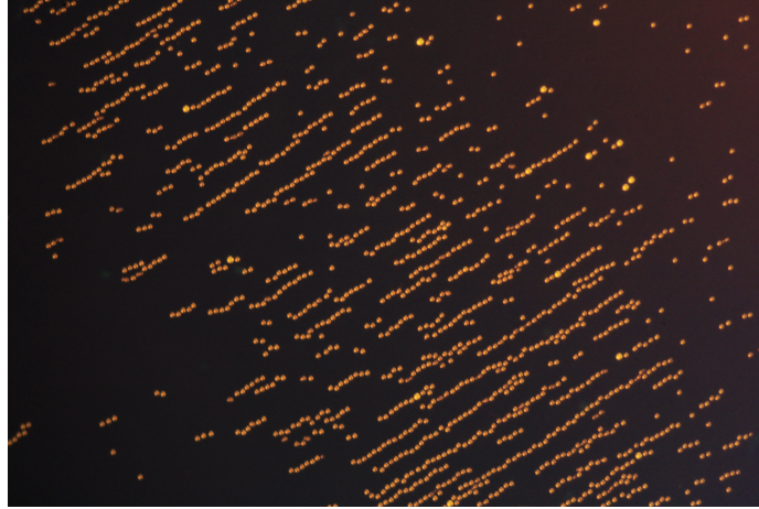
Figure 4.2: "Magnetic holes" aligned into particle chains by an in-plane external magnetic field. The particles are non-magnetic spheres with diameter 40\ \mu\text{m} , but they are suspended in a ferrofluid. Own work from last year's master's project.
