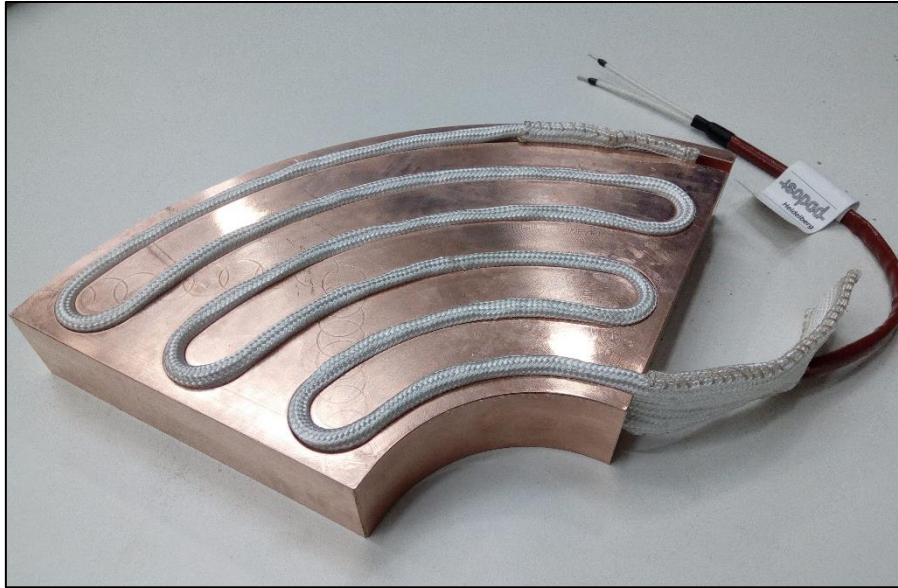
Figure 3-6: Finished heating plate with inserted heat cable
