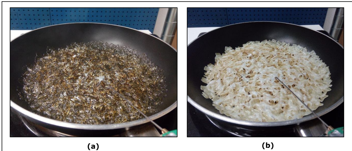
Figure 4-3: Colour change in HDPE without thermal oil; (a) at melting temperature; (b) solidified at room temperature
