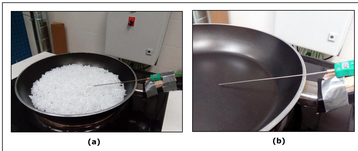
Figure 4-1: Preliminary test set-up; (a) frying pan with HDPE shavings; (b) thermocouple placement
