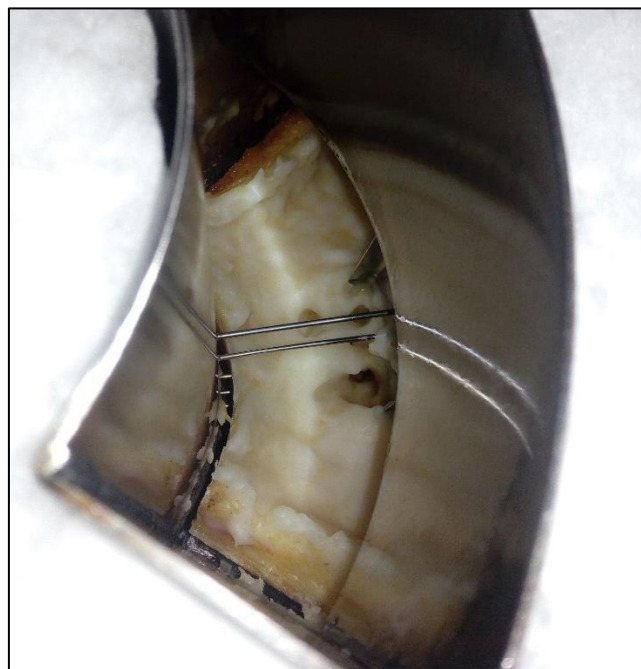
Figure 4-8: HDPE shavings melted into a solid lump
