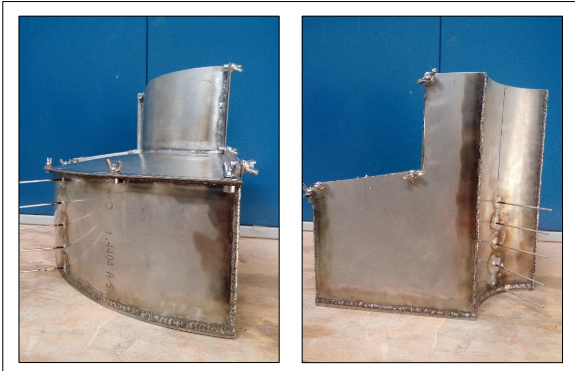
Figure 3-4: Finished container with cannula pipes
