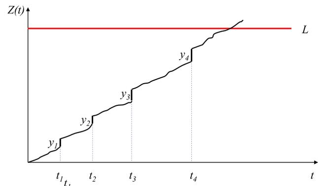
Fig. 2. The degradation behavior of one unit based on the two processes.
