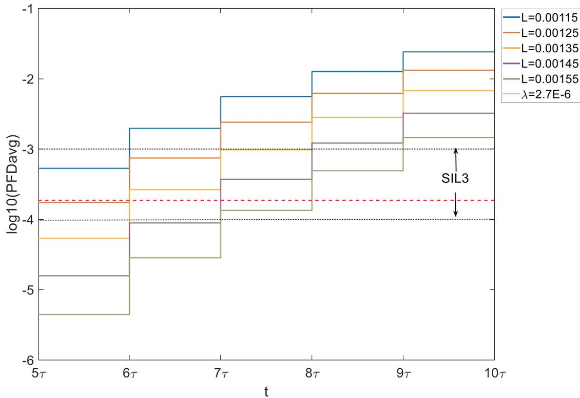
Fig. 6. Effects of threshold  $L$  on  $PFD_{avg}$ .
