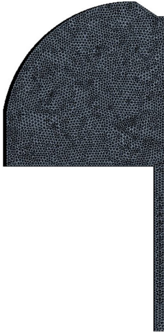
Figure 9.2: Mesh with 200 mm grid size used for the CFD simulations (symmetrical plane)
