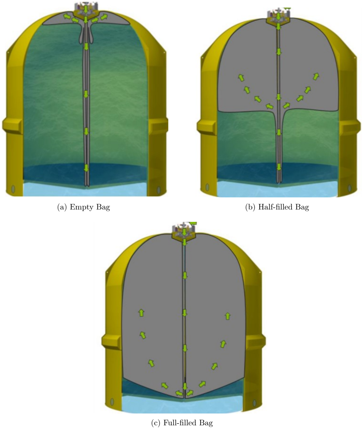
Figure 3.3: Filling sequence of the bag illustrating the downward movement of the bag and outward displacement of the sea water as oil fills the bag [15].
