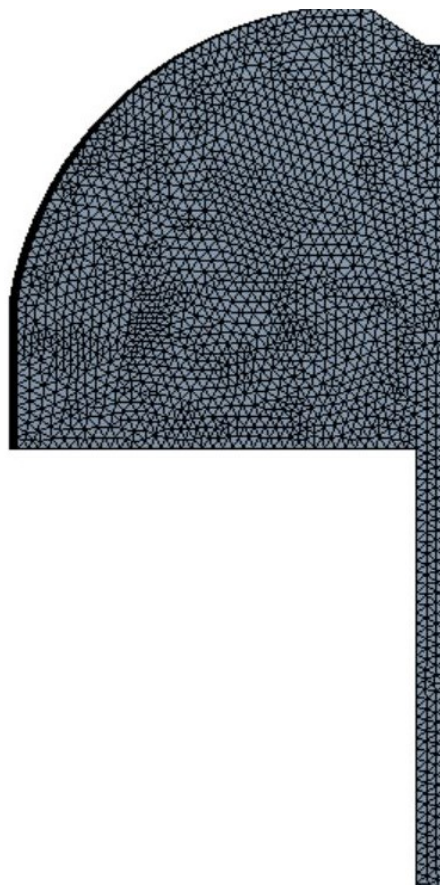
Figure 6.5: Initial Mesh of Fluid domain with 300 mm mesh size (symmetrical plane)
