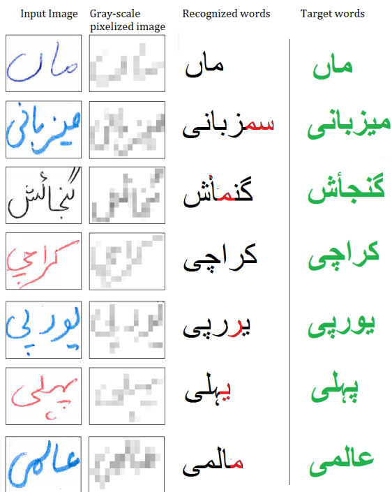
FIGURE 10. The original images are presented with their corresponding pixelized gray-scale images. The misclassified characters are represented in red color whereas, the target words are represented in green text.
