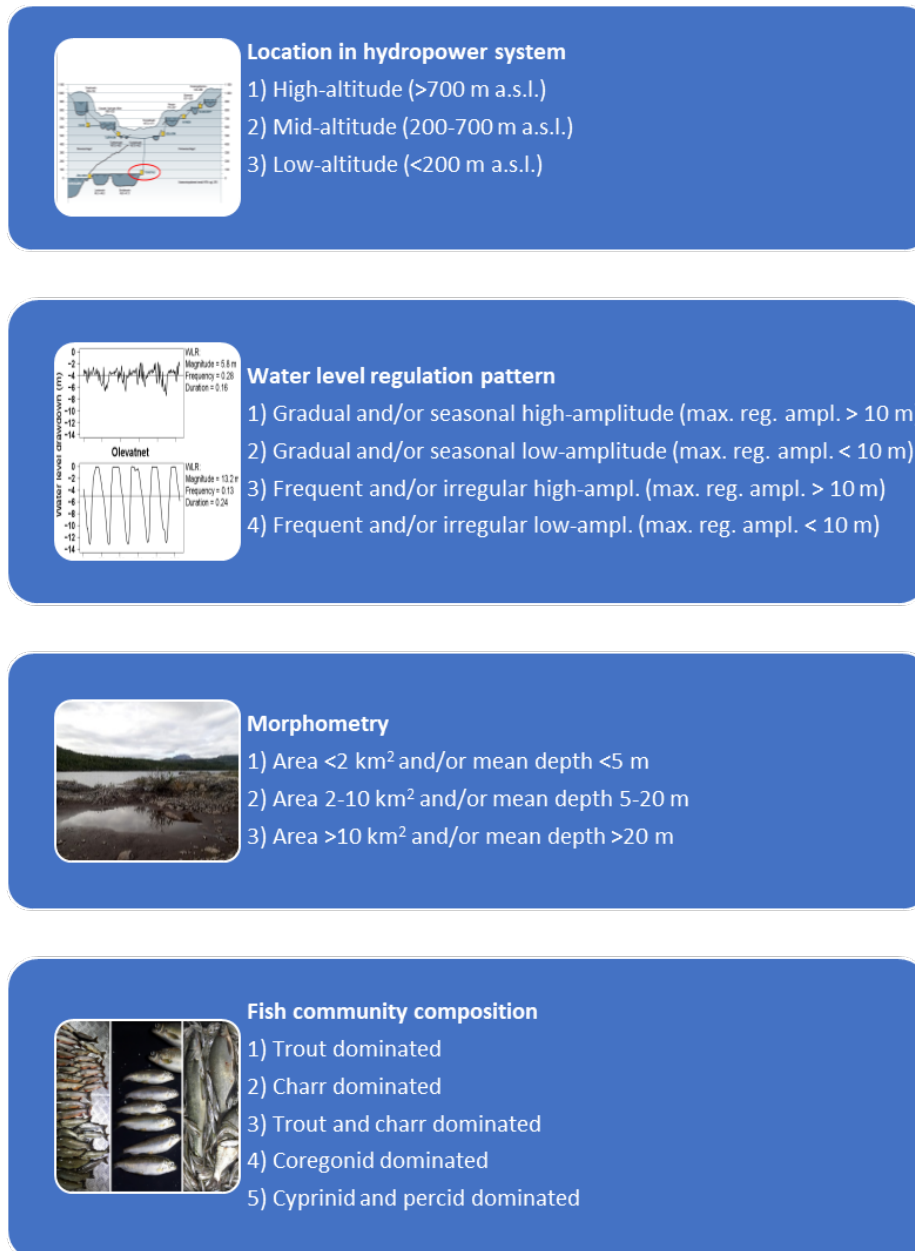
Figure 9. Suggested examples of classes describing some important abiotic, biotic and hydropower-related characteristics for Norwegian hydropower reservoir. The list is just an illustration of a conceptual way of defining different reservoir types and should not be understood as a final suggestion for a categorization system for Norwegian hydropower reservoirs.
