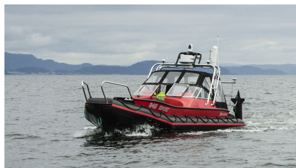
FIGURE 3 The Telemetron ASV, designed for both manned and unmanned operations. Courtesy of Maritime Robotics [Color figure can be viewed at wileyonlinelibrary.com ]
