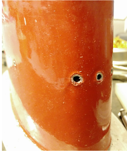
Figure 28: Coated foil with rough edges around the sensors' measuring points.
