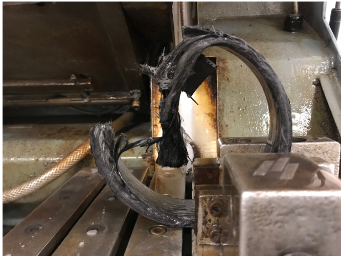
Figure 4.10: A poorly impregnated composite left completely destroyed by the cutting process
