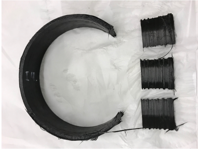
Figure 4.9: Appearance of a dry composite after cutting
