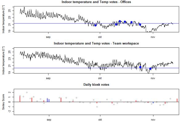
Figure 4. Time series plot of Space 2. Top two plots show temperature at 15 minute intervals in offices and open team workspace. Blue dots where occupants have made a digital complaint about "Too cold". Red dots where complaint "Too hot". Red and blue lines as "mean complaint temperature for hot and cold. Bottom plot shows 2-day mean of satisfaction votes (circles) from "Angry" = -2 to "Happy" = 2. Red bars are weekly mean, blue bars are monthly mean.
