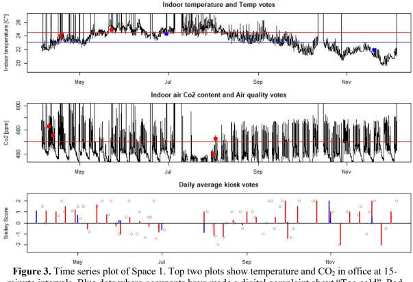
Figure 3. Time series plot of Space 1. Top two plots show temperature and  $CO_2$  in office at 15minute intervals. Blue dots where occupants have made a digital complaint about "Too cold". Red dots where complaint "Too hot" and "Bad air in middle plot. Red and blue lines are mean of dots. Bottom plot shows 2-day mean of satisfaction votes (circles) from "Angry" = -2 to "Happy" = 2. Red bars are weekly mean, blue bars are monthly mean.
