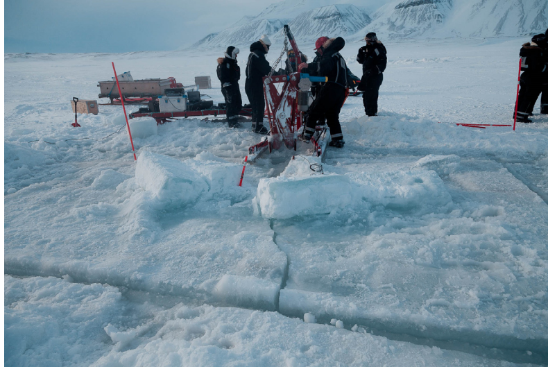
Figure 8. After the ice ridge splitting test.
