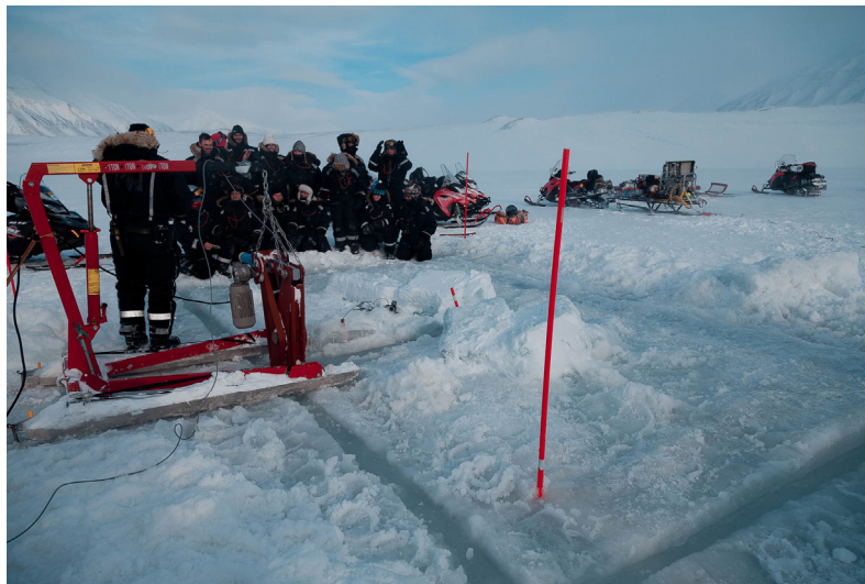
Figure 7. Artificial ice ridge splitting test.
