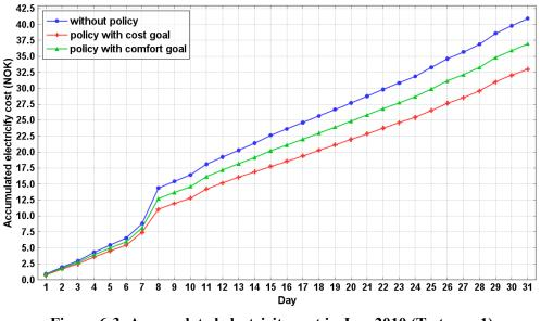
Figure 6-3: Accumulated electricity cost in Jan. 2010 (Test case 1)
