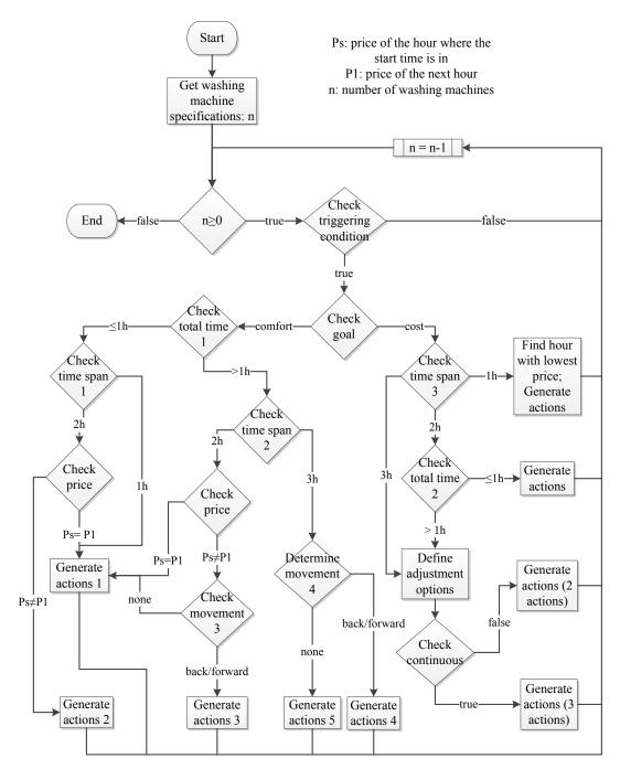
Figure 5-3: Policy logic for the washing machine model
