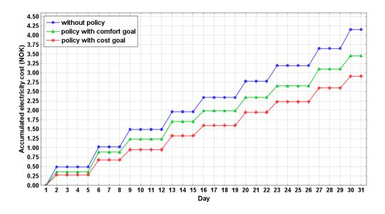
Figure 6-7: Accumulated electricity cost of the washing machine (Test case 1)
