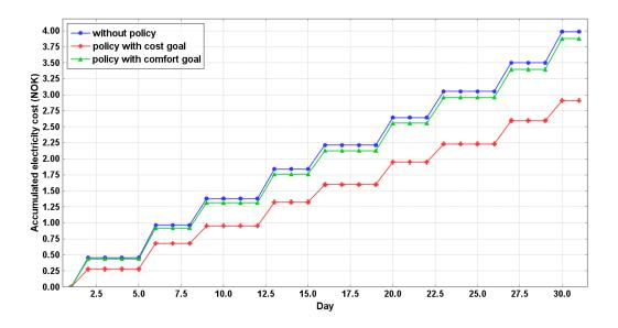
Figure 6-9: Accumulated electricity cost of the washing machine (Test case 3)
