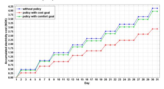
Figure 6-8: Accumulated electricity cost of the washing machine (Test case 2)
