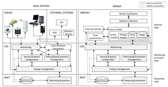
Figure 3-1: Functional architecture of the real system vs. SMASH 37 [12]
