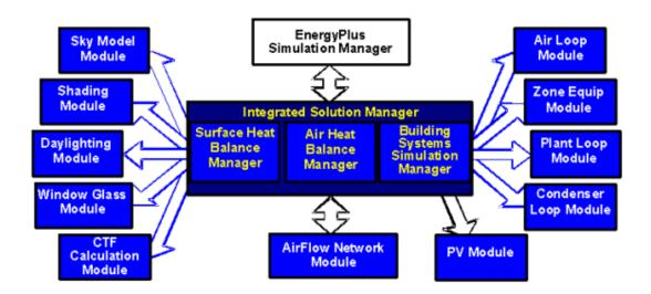
Figure 2-2: Integration of elements of a building energy simulation [9]
