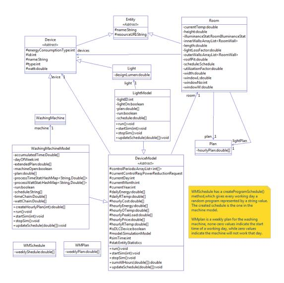
Figure 5-1: Class diagram for the implementation of energy models
