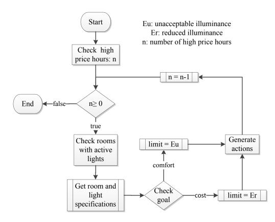
Figure 5-2: Policy logic for the lighting system model
