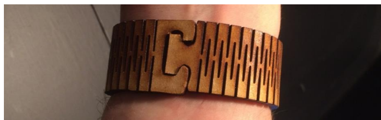
Figure 5: Wristband made of MDF using pre-made living hinge patterns.
