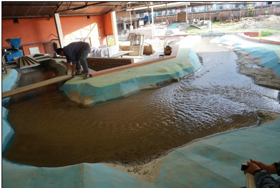
Figure 3-1 A river model without hydraulic structures (Photo: Hydro Lab)
