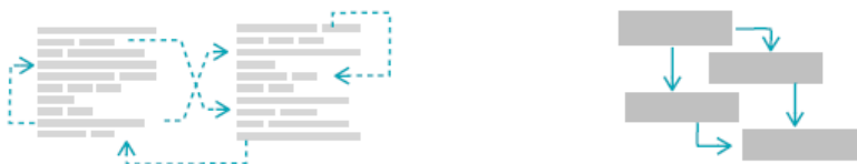
Figure 2.8: The flow of a program is illustrated, where the left side shows code, and the right side shows graphical building blocks. The dotted arrows would not be visible in most editors. Image from http://reference.bitreactive.com/papers/secret-twists.html
