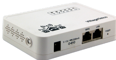
Figure 2.2: The second generation Mesh Potato, MP02.
