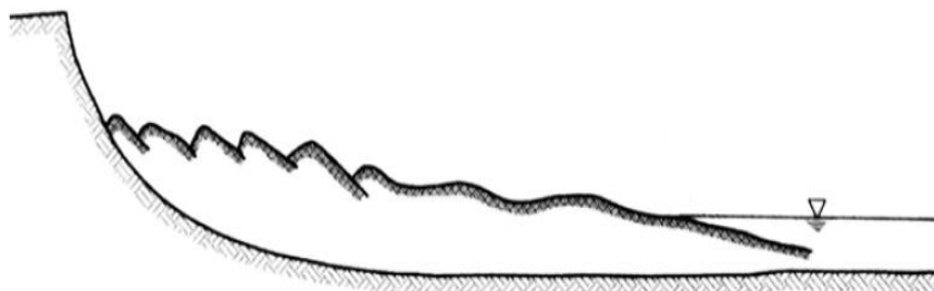
Figure 2.13 Slope failure in unconsolidated silt and clay (Morris and Fan, 1998).
