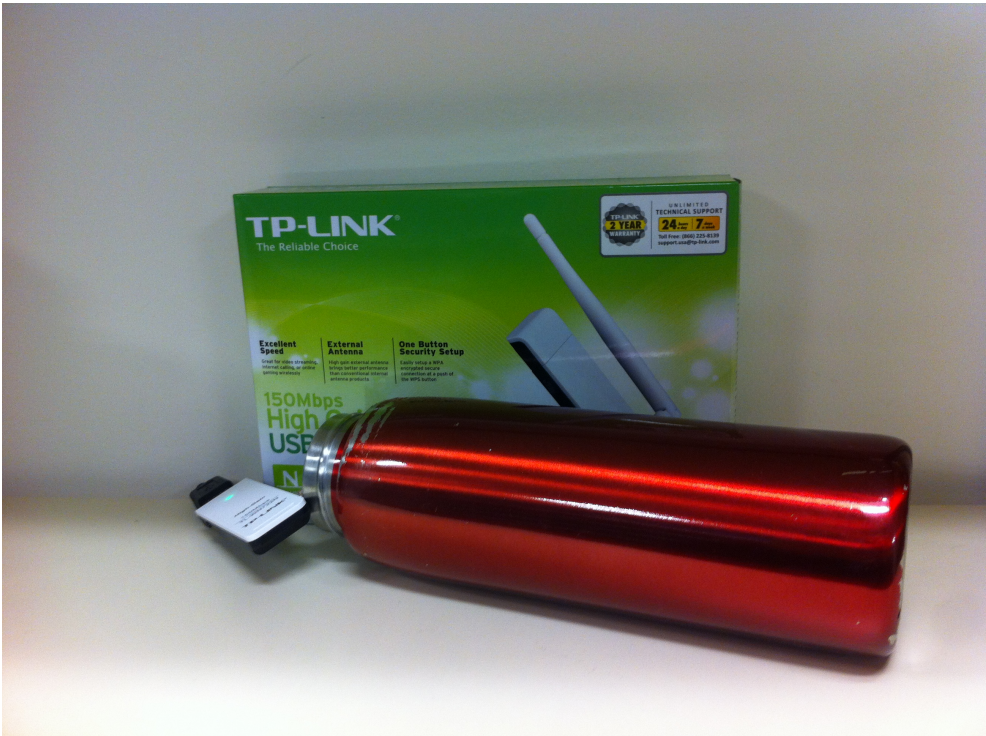
Figure 3.9: Description of how attenuation of signal is achieved, and consequently packet losses.
