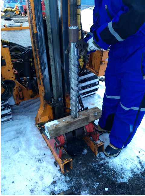
Figure 5.3: The drill rig with the CRREL barrel for drilling in frozen soil.
