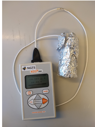
Figure 5.6: The KD2 Pro device and TR-1 sensor inserted in a soil sample wrapped in cling film and aluminium foil.
