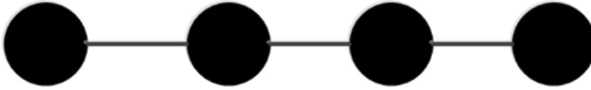
FIGURE 15: TOPOLOGY 2 - A CHAIN OF NODES
