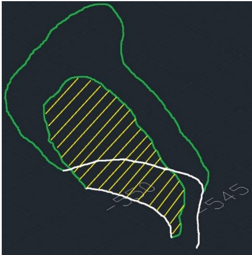
Figure 14: The white lines are the original contours, the green the new contours and the area (marked with yellow lines) multiplied with the contour difference can give a volume approximation.
