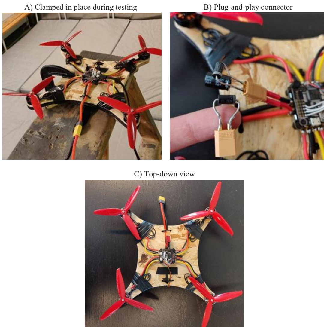
Figure 3.1: “Woody” test platform. The ESC and flight controller are stacked in the center.
