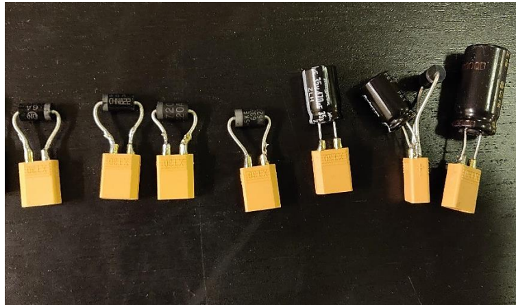
Figure 4.6: Example of components made for testing. They included single TVS diodes, capacitors and combinations of them in parallel.
