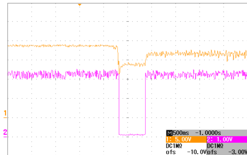
Figure 5.13: Stepping from low to high rpm with the active battery interface installed.
