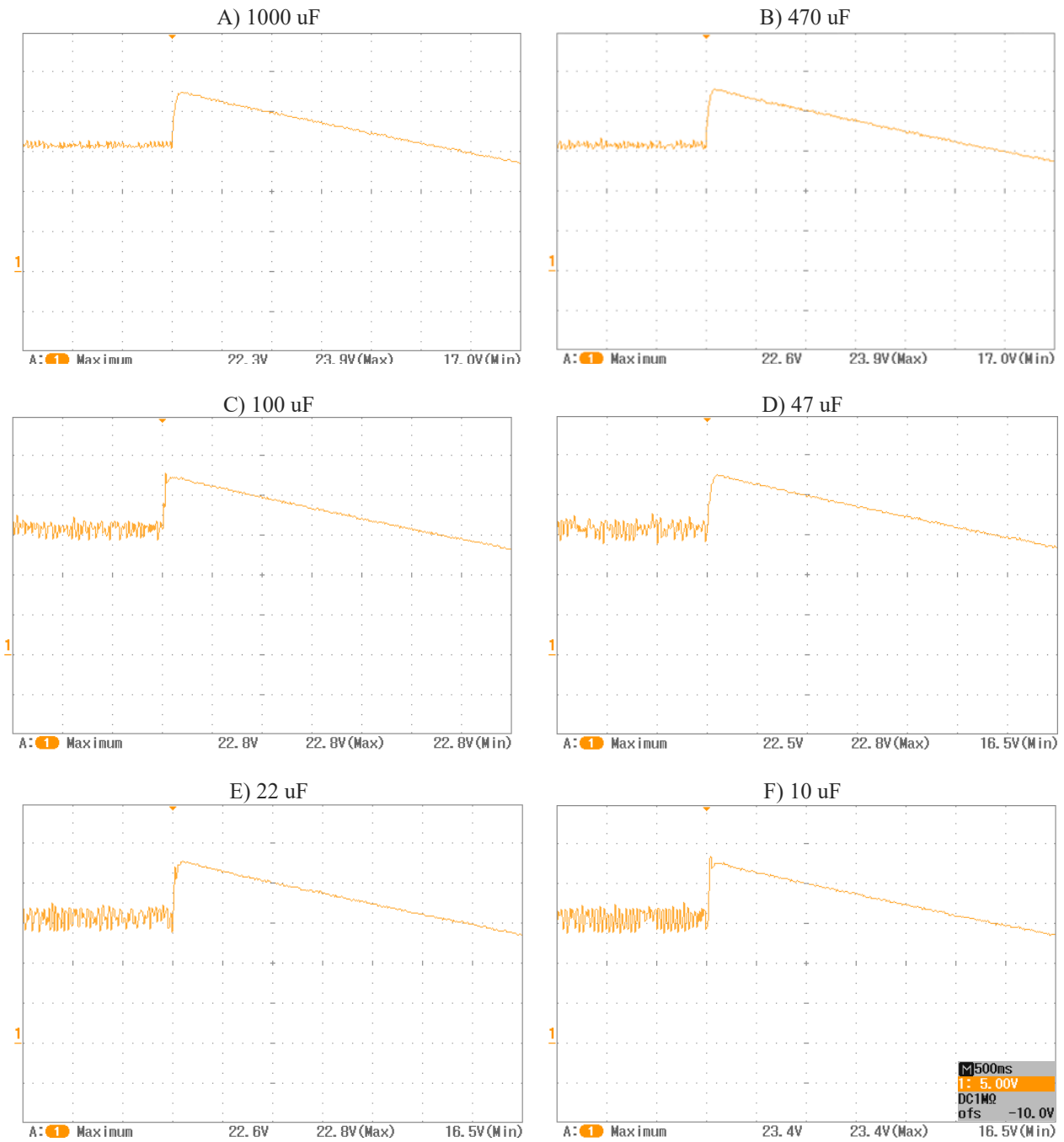
Figure 4.10: Smaller valued capacitors at 80 % thrust on 16.5 V / single 1700 Kv.
