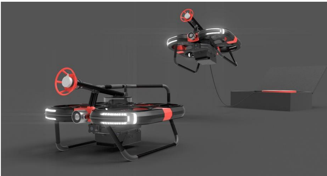
Figure 1.1: A conceptual rendering of a Scout Drone Inspection quadcopter. The drone in the back is flying on a tether.
