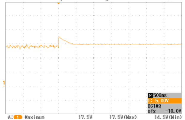
Figure A.3: Combinations of 16 V TVS diodes and 470 uF in parallel at 60 % on 15 V / Woody.
