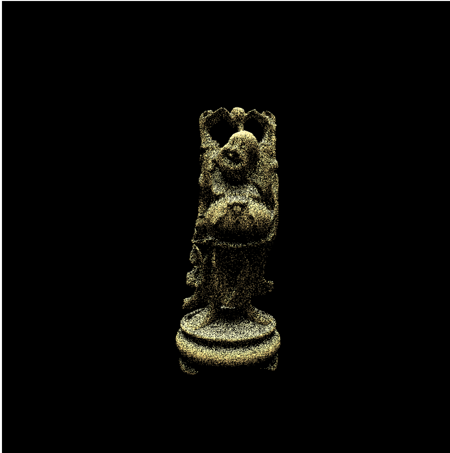
Figure 3.1: budda.brhan rendered with 1 SPP (model courtesy of Stanford Computer Graphics Laboratory[35] via PBRT scenes[36]).
